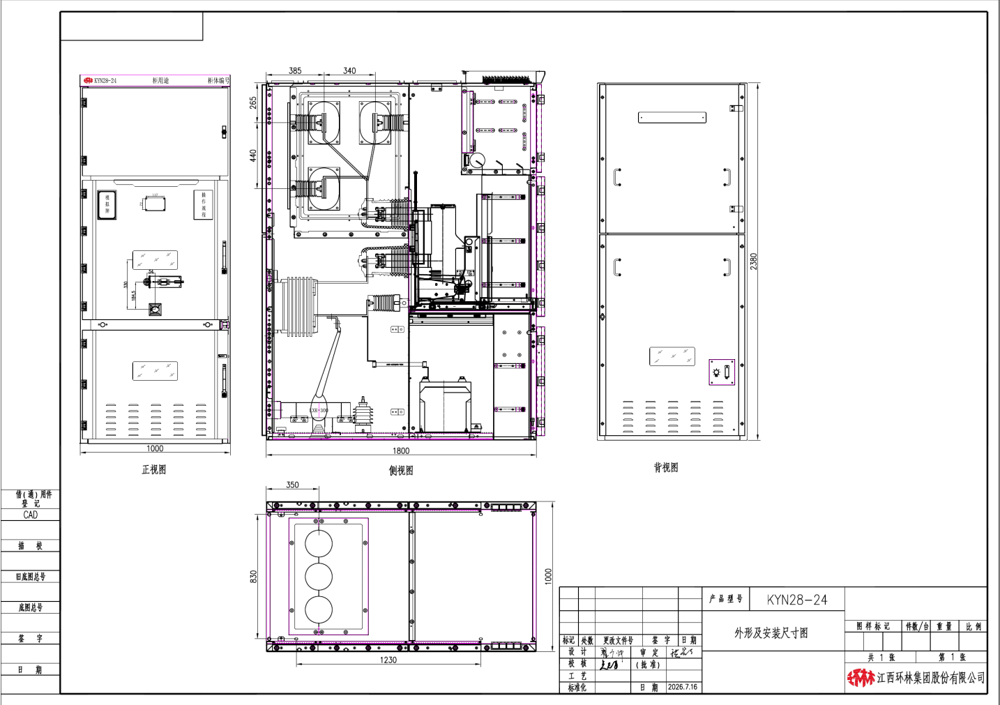
Fig. 2 — KYN28-24 Outline and Installation Dimensions
